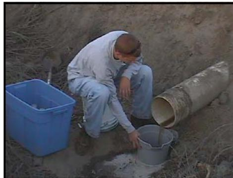
Tail water discharge being measured using bucket method.
